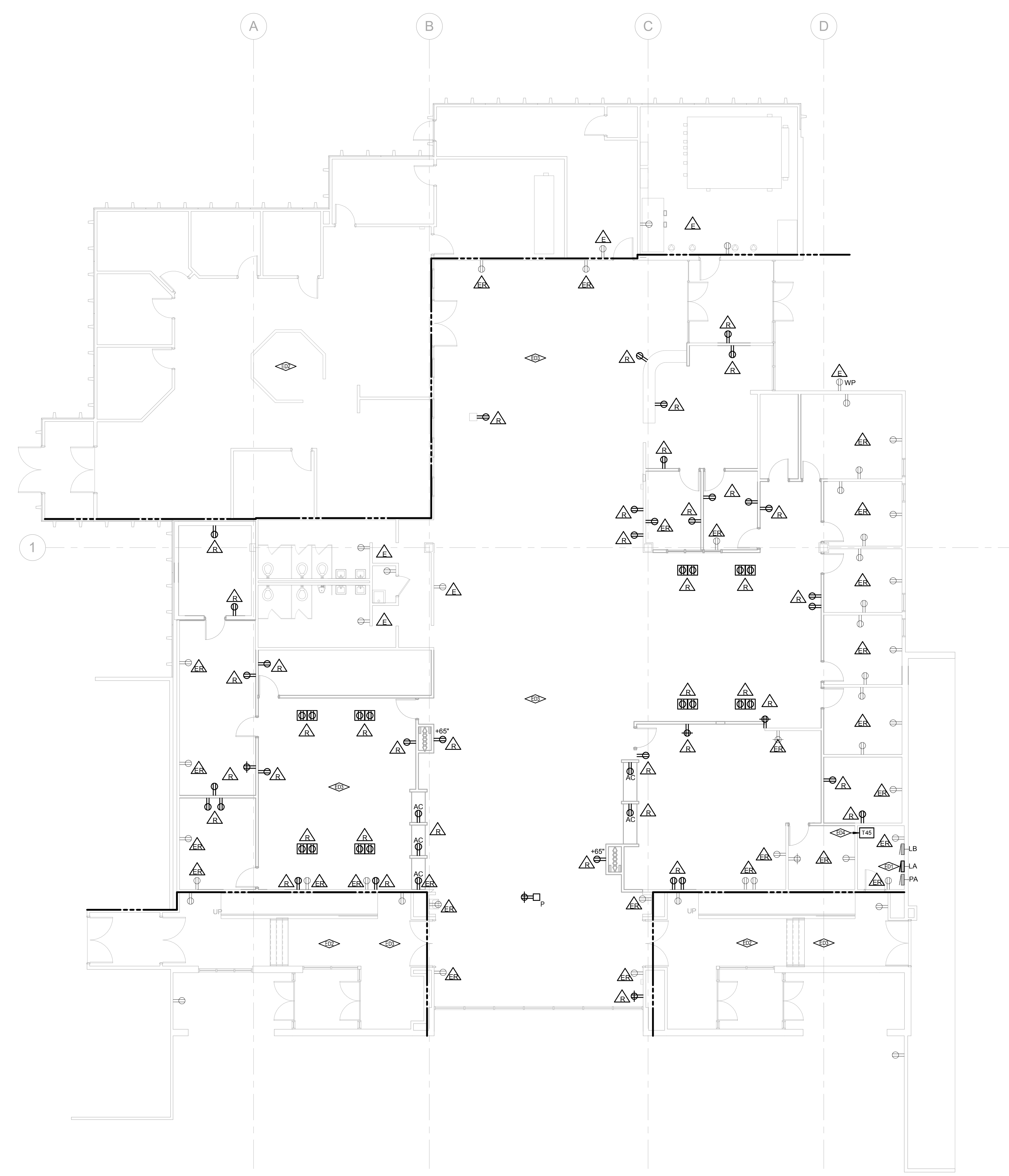
↑ FIRST FLOOR POWER/FA DEMOLITION PLAN SCALE: 1/8" = 1'-0"
