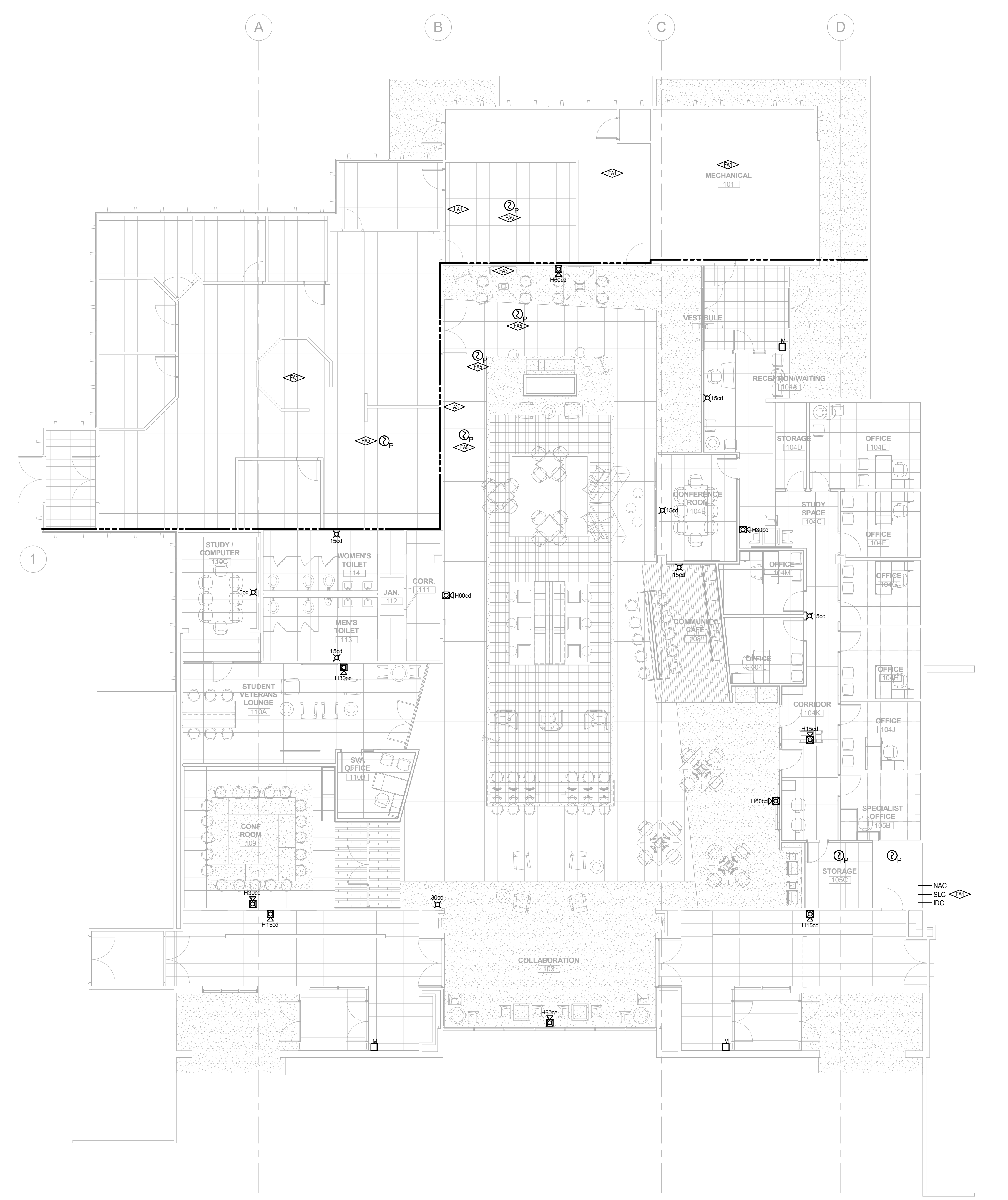
FIRST FLOOR FIRE ALARM PLAN SCALE: 1/8" = 1'-0"
