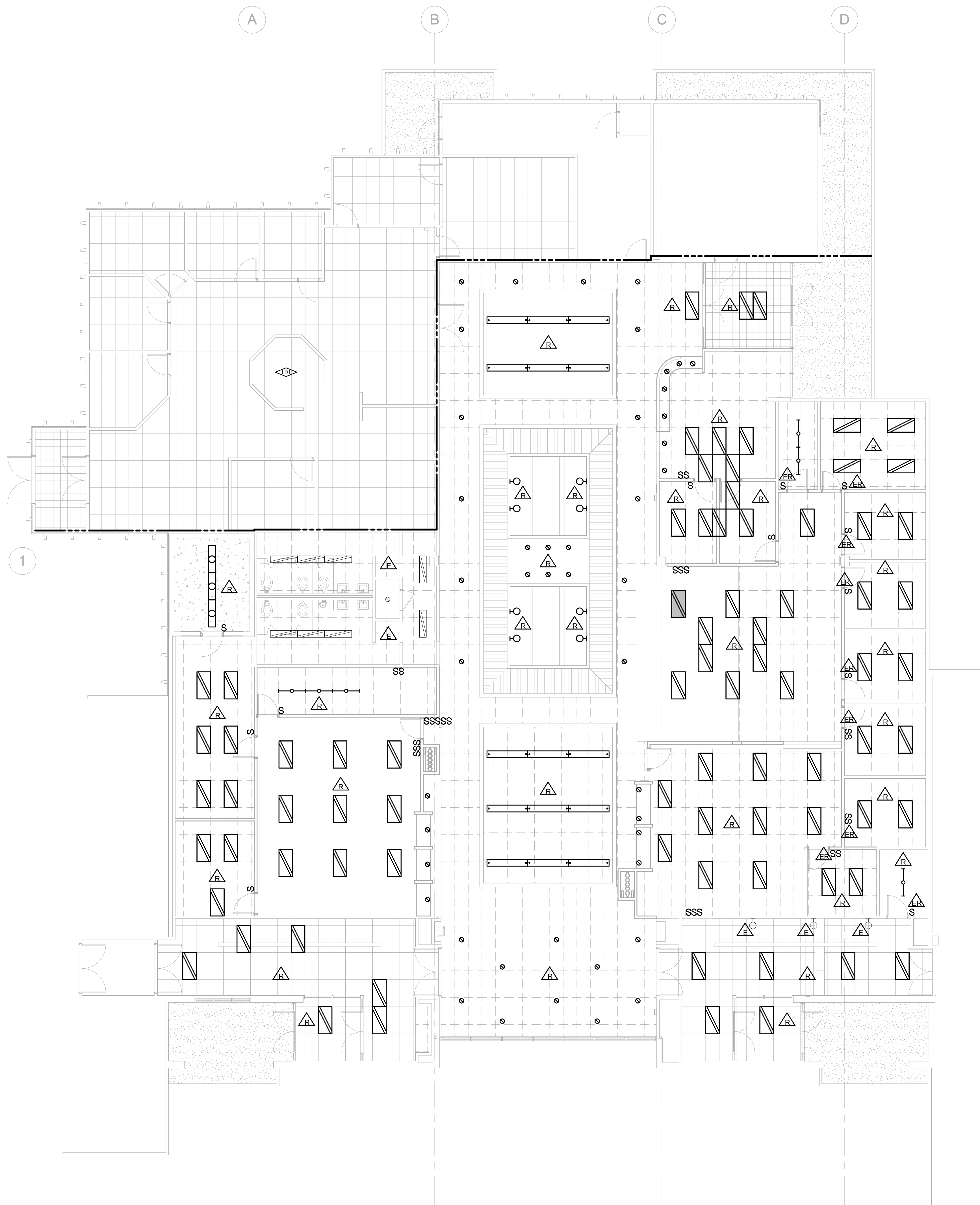
FIRST FLOOR LIGHTING DEMOLITION PLAN SCALE: 1/8" = 1'-0"
